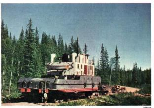
The Radium Franklin is portaged around rapids in upper Bear River. She is one of a new fleet designed especially to carry uranium ore
